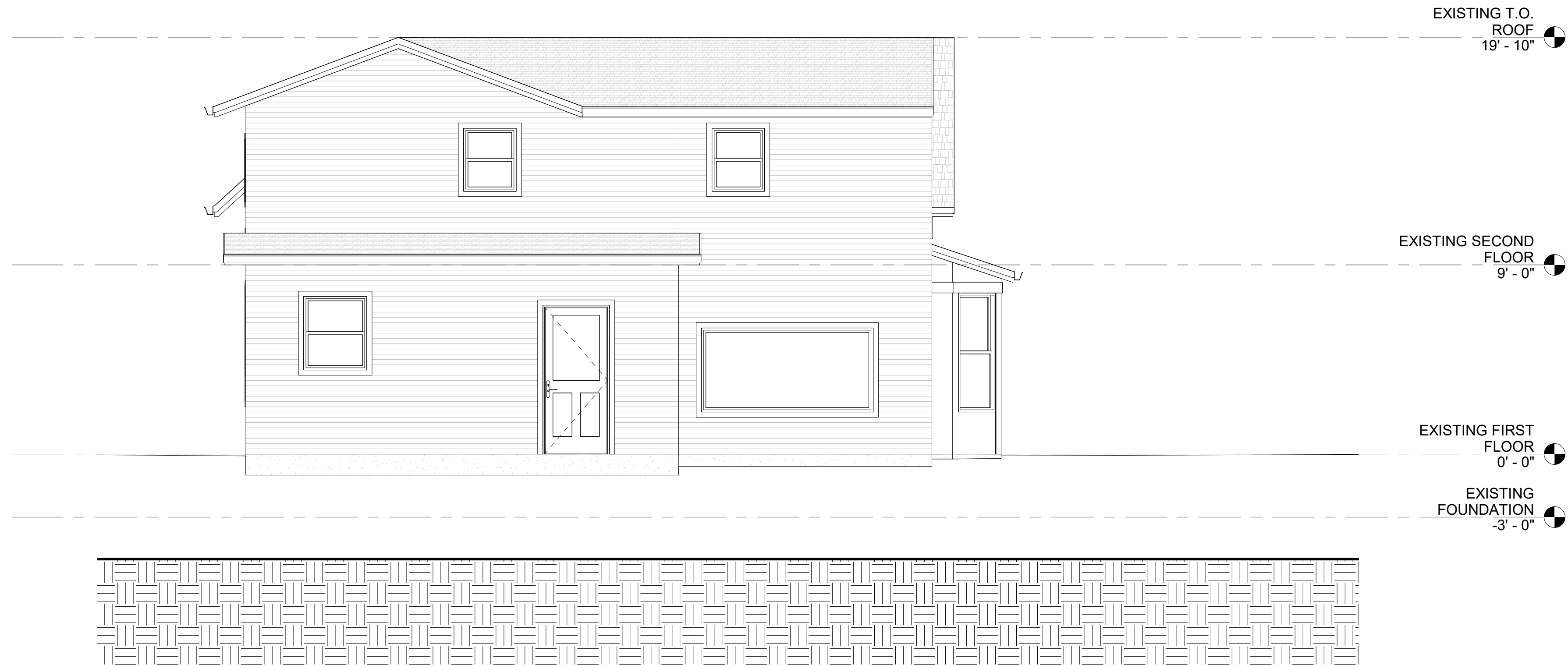
② EXISTING WEST ELEVATION 1/4" = 1'-0"
