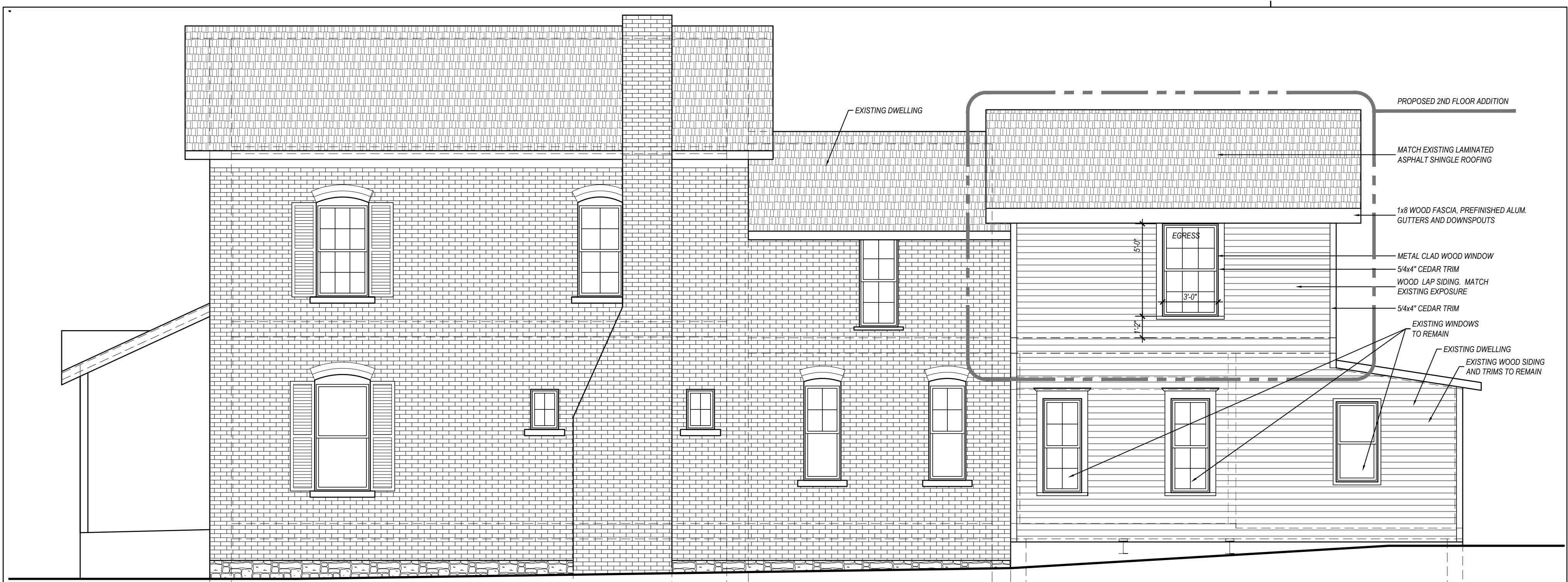
1 PROPOSED NORTH ELEVATION 1/4" = 1'-0"
