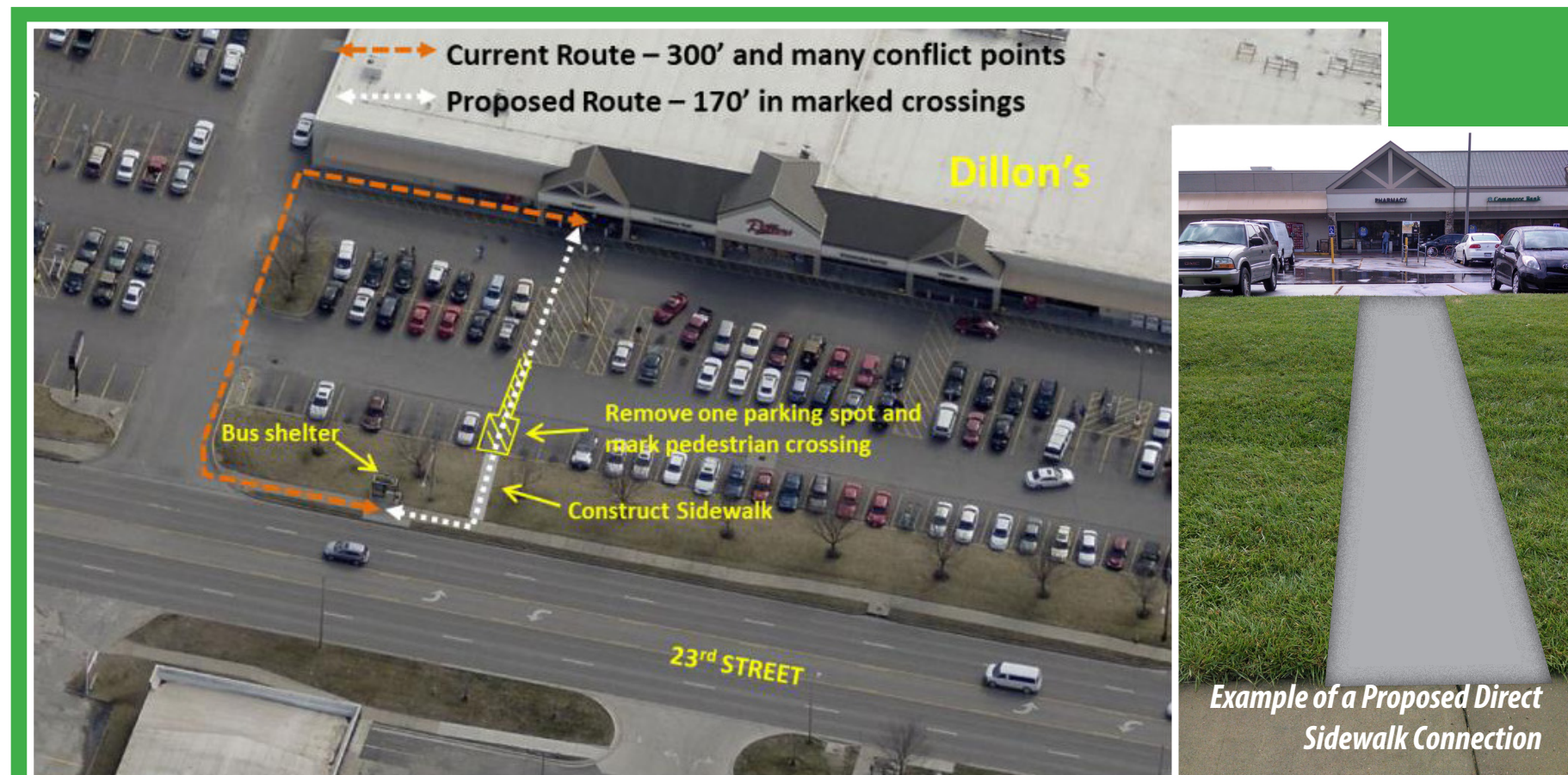
Figure 5-5: Examples of Pedestrian Connectivity Issues between Bus Stop and Development
