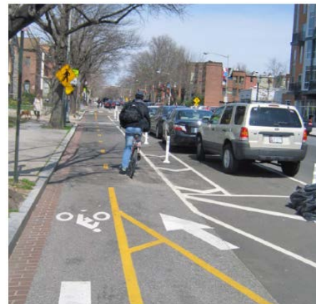
Figure 8: Example of Cycletrack (Protected Bike
