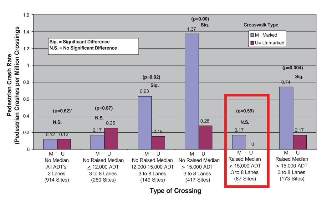
Figure 4. Pedestrian crash rate vs. type of crossing.
