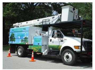
The new boom truck that is also green, as it uses a hybrid system and provides full electric stationary operation of the bucket truck, eliminating the use of diesel fuel to operate the bucket lift system.
