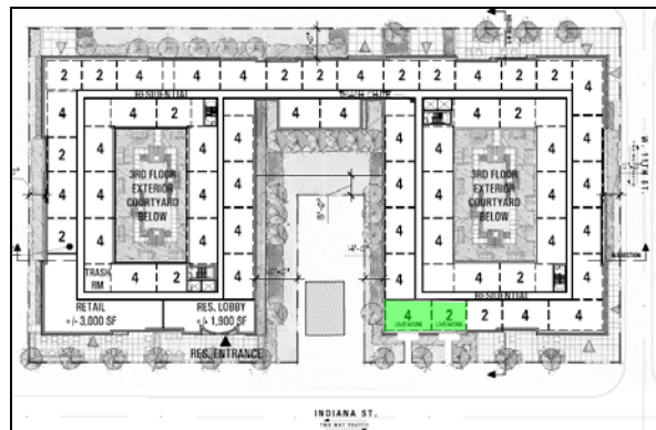
Figure 3 Fourth Floor Plan Showing Work Live Units
