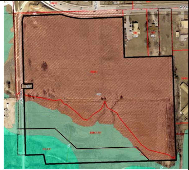
Figure 2. Regulatory floodway and floodway fringe, shown in dark and light green, and the FP Overlay District north boundary in red.
