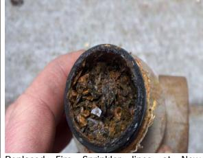
Replaced Fire Sprinkler lines at New Hampshire Parking Structure
