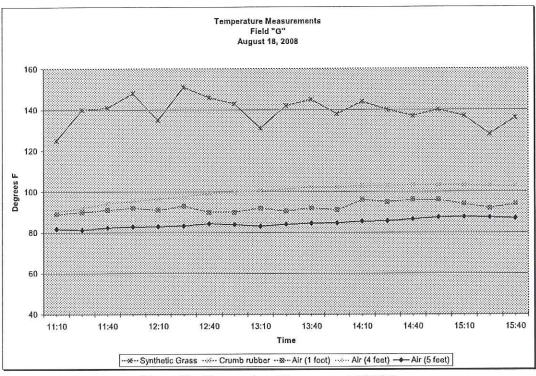
Figure 11 - Temperature Measurements Field G
