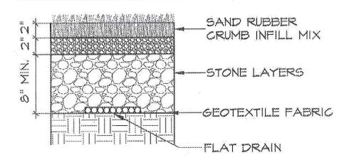
Figure 3 - Typical Field Cross Section
