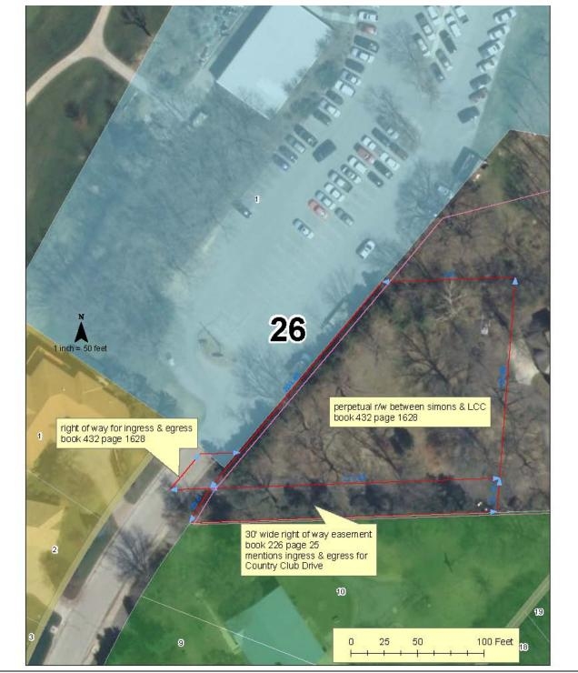
**Figure 3.** GIS map showing the location of the right-of-way, right-of-way easements, and property lines. The colored properties are platted, with each color being a different plat.
